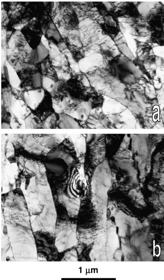
Fig. 7. Micrographs showing microstructure in unirradiated materials of (a) the TS-tube and (b) the ITS-specimen of LiSoR-2.
